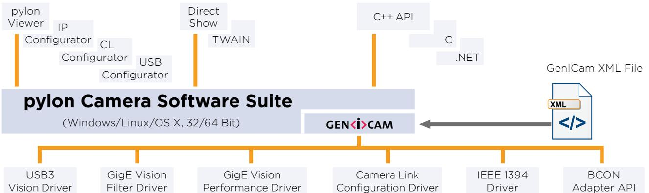
The architecture of the pylon Camera Software Suite is based on GenICam Technology, which offers you easy access to the newest camera models and the latest features. Changes to an existing camera device in your application essentially become a plug-and-play process.
