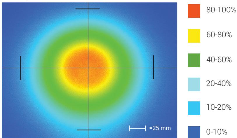
Optical measurement taken using SL112-WHI @ 300 mm
