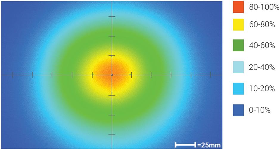
Optical measurement taken using SL-S050075M-WHI @ 300 mm
