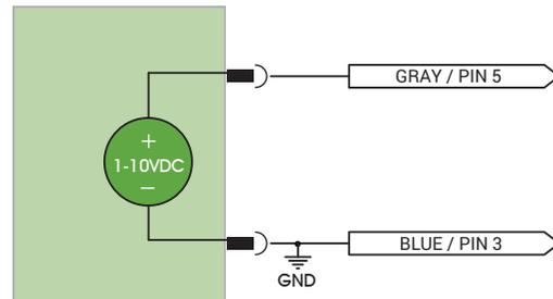
Analog dimming works in both strobe and continuous
