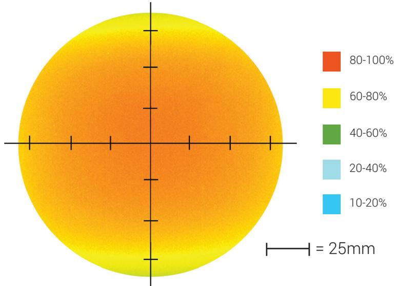
Optical measurement taken using DL067-WHIIC @ 25mm
